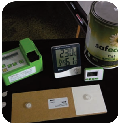
One week later, formaldehyde emissions were tested with Yangisawa Sensors and Flux Monitor. Emissions can be read via either Desiccator (mg/L) or Small Chamber ( \mu\text{g}/\text{m}^2/\text{hr} ) methodology.
