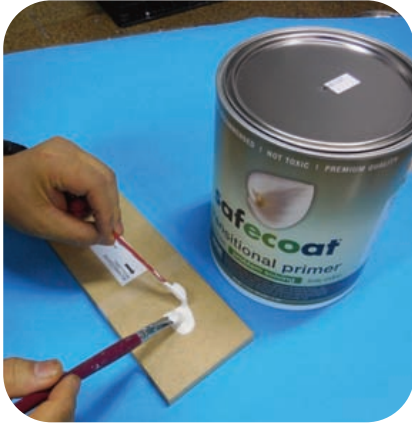
Primer was applied with 1.2ml / 0.01 sq.mtr (which is equivalent to 336 sq.ft/gal)
